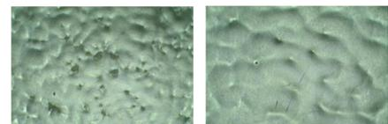
*Photo: conventional anilox smoothness (left) & GTT smoothness (right)*
